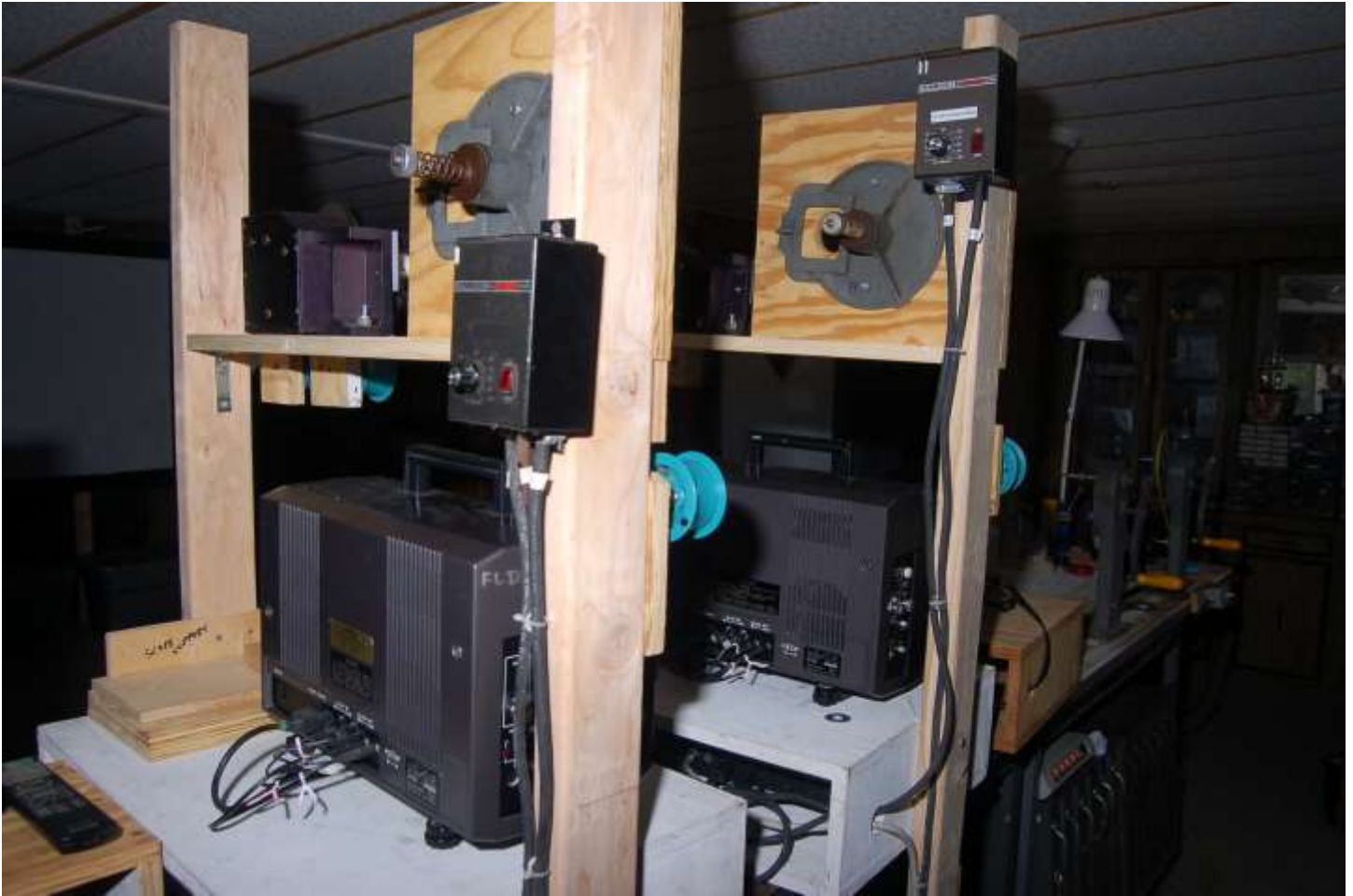
The back side of the Towers. Baldor speed controllers model BC138. The different placements were to find out which height is better. I'm going with the one on the right.
