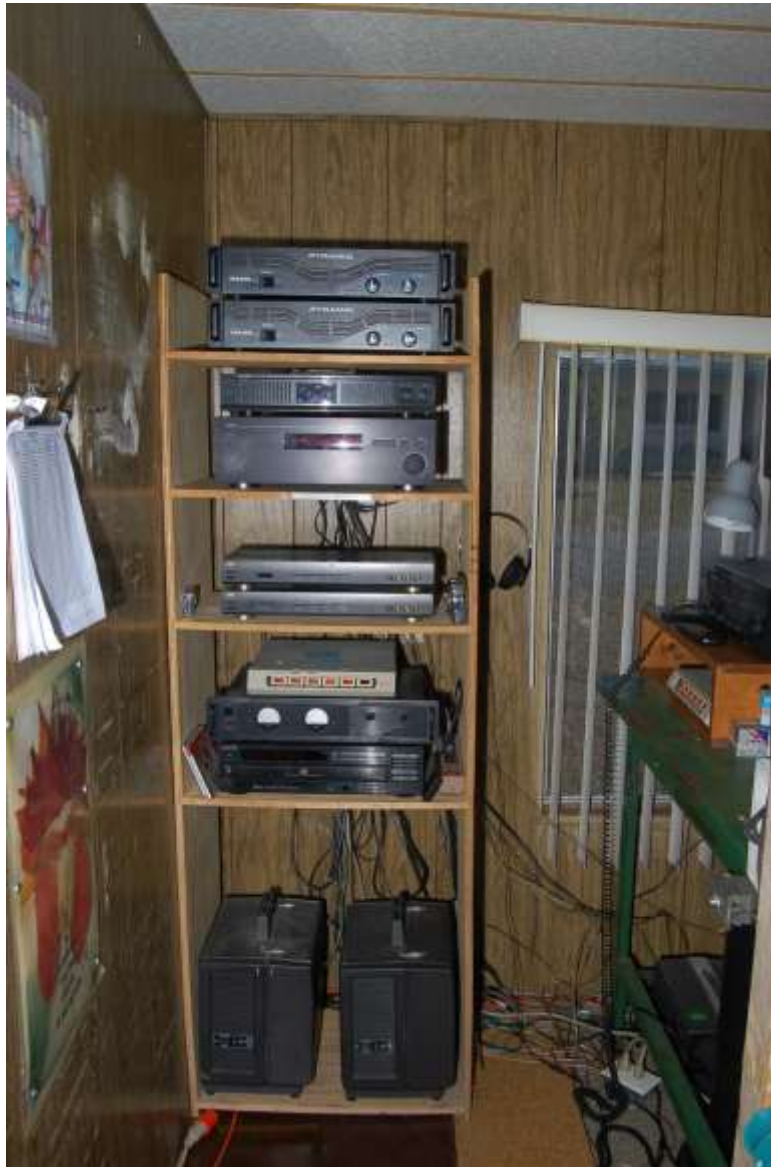
Cinema sound system. 1200 watts of power. L C R + Subwoofers (2) @ 250 per channel Rear Surrounds @ 100 watts per channel Subwoofers are tied into the right channel only of the 2 nd stronger amp That shares the left channel with center. Left and Rights are equalized.
