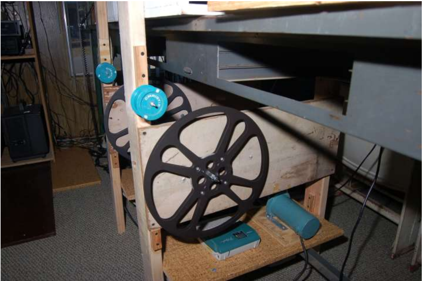
The bottom of the Towers. Super 8 Goldberg reels @ 2000 foot. 35mm Christie Platter AW3 parts. Rollers & drive motor. Deluxe double drawer Neumade rewind bench.
