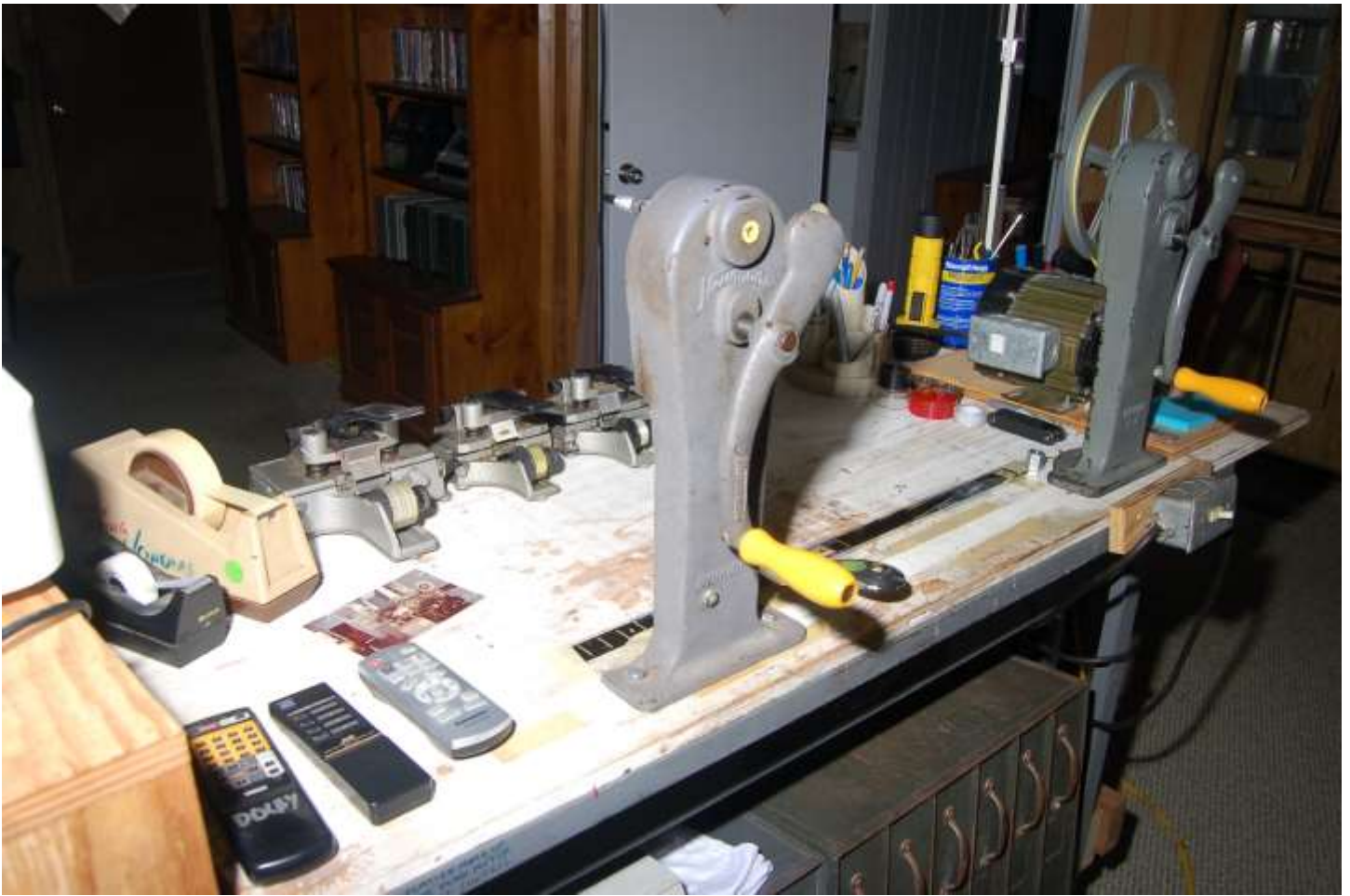
Top of rewind bench. Neumade X-3 rewinds with motor and pulley for 35mm. Customized adapters to the 5/16 shafts for super 8 & 16mm.
