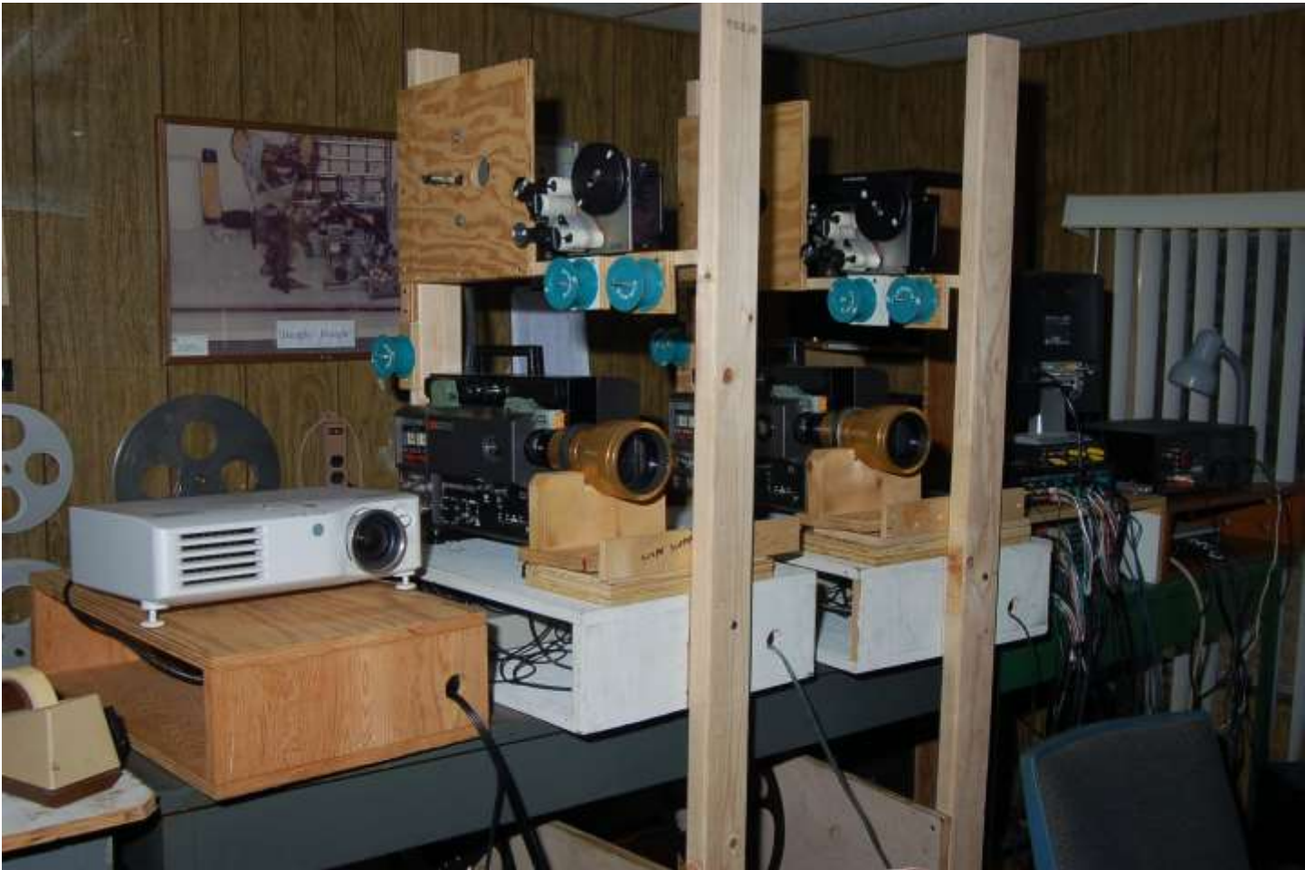
Two brand new Towers. Dual format for super 8 and 16mm. GS 1200 projectors and the Panasonic AX-200-U.
