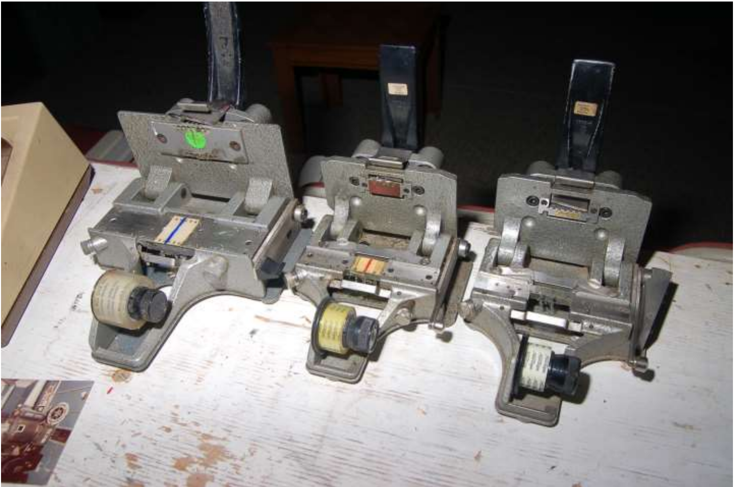
Ciro Guillotine M-3 Special splicers. Left to right: 35 / 16 & reg 8 / super 8 These are my favorite splicers and the Best ones I've ever owned. The official model number is "M-3 Special" Plus the format you need.
