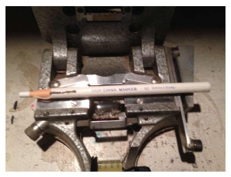
A China marker or also called a Grease pencil can be used to make the white lines on countdown leaders. Be certain to be marking between magnetic tracks with the sound tracks in the UP position. As the soundtracks face the lamp house in the top loop of the projector.
