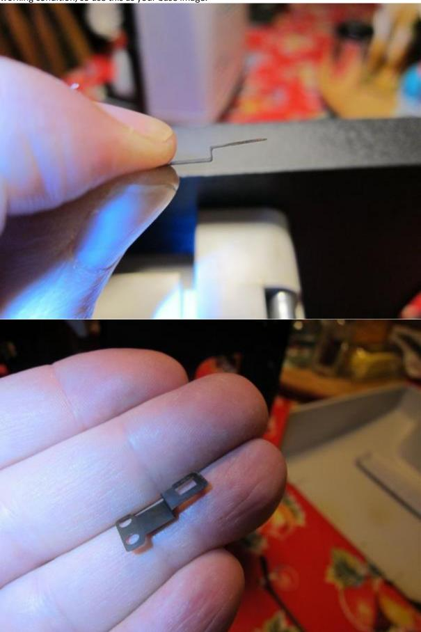
The flat parts should be PERFECTLY FLAT, and the zig-zag "bend" should be such that when the holding screws to this aperture are tightened down, the flat opening slides PERFECTLY FLAT against the larger S8mm opening. You can see it when you see it.
